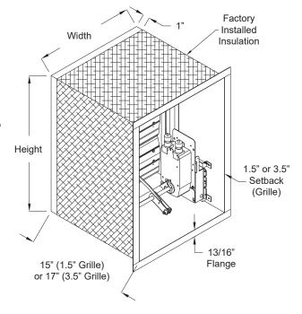
Combination Fire/Smoke Damper ▲ 1½ Hr. Rated ▲ Airfoil Blades ▲ Leakage Class I ▲ 250°F or 350°F Rated ▲ Out-of-Barrier ▲ Galvanized Steel
